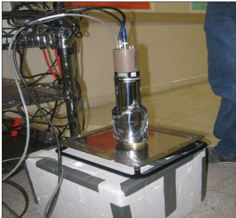
Figure 3.- Spectroscopy system to measure a wedge.
