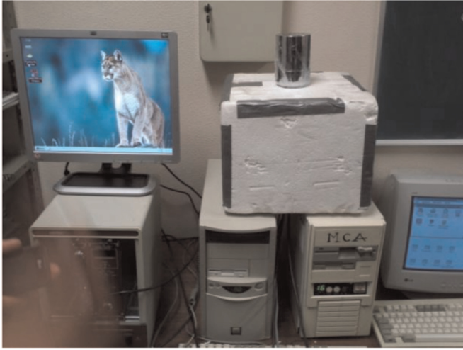
Fig. 2. Gamma-ray spectrometer with a 7.620 \times 7.62 \text{ cm}^2 NaI(Tl) detector.
