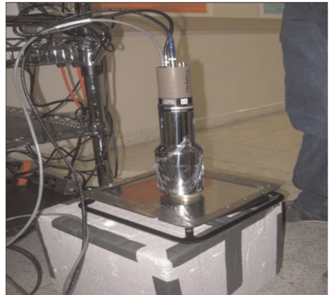
Fig. 5. Spectroscopy system to measure a wedge.
