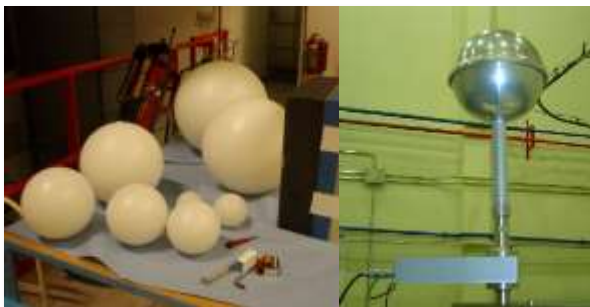
Figure 4. The UAB BSS. At the right, the 4.2" sphere with cadmium shell during measurement.
