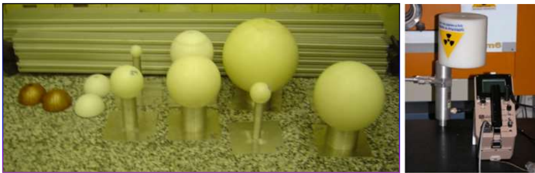
Figure 3. The INFN BSS: bare, 2", 3", 5", 7", 7"+Pb (4" int. diameter, 1/2" lead), 8", 10", 12", 12"+Pb (8cm int. diameter, 1cm lead). Polyethylene density 0.95\text{ g}\cdot\text{cm}^{-3} . At the right, the reproducibility check device.
