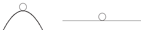
Figure 3. A system in unstable and neutral equilibrium: a schematic representation of the key phenomena underlying the two concepts of inertial frames.
