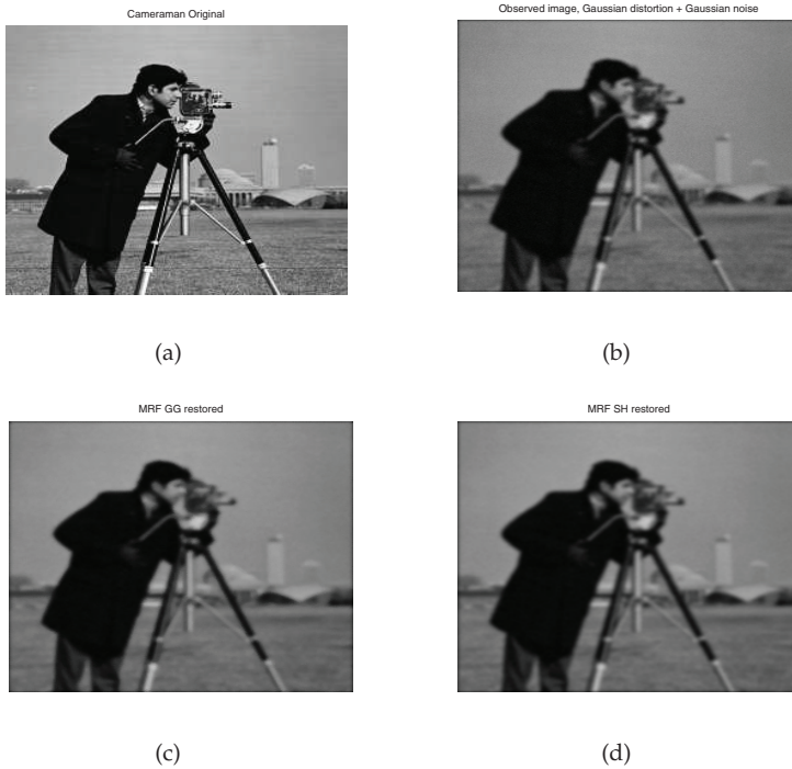
Fig. 4. Results for Cameraman standard image: (a) describes the original Cameraman image; (b) describes the distorted image using Gaussian noise with \sigma_n = 3 ; (c) partially restored image using MAP1 ( \lambda = 30, p = 1.2 ); (d) partially restored image using MAP2 ( \Delta_0 = 20 ).
