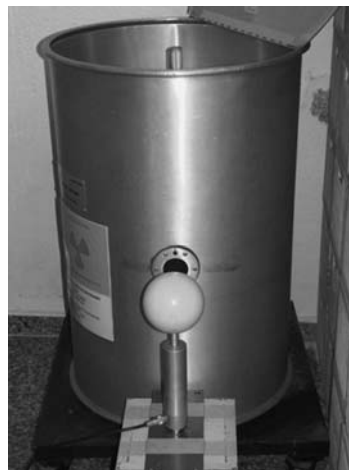
Figure 1. Image of the neutron Howitzer container with a Bonner sphere aligned with the irradiation tube.
