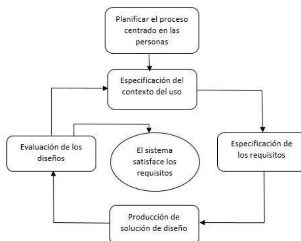
Fig. 2. Estándar ISO: 9241-210:2010, Ergonomics of human-system interaction, part 210 Human-Centred Design for Interactive Systems [4].
